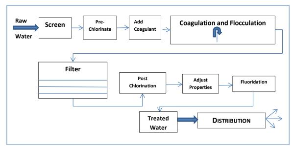
Figure 3: Water Filtration Plant
