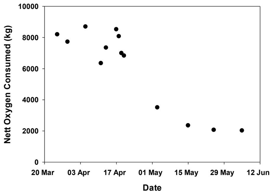
**Figure 1:** Nett oxygen consumption over time in Weir 32 weir pool in the reach between the Lake Pamamaroo outlet and the lake Menindee outlet. Nett oxygen consumption was calculated from WaterNSW longitudinal surveys.
