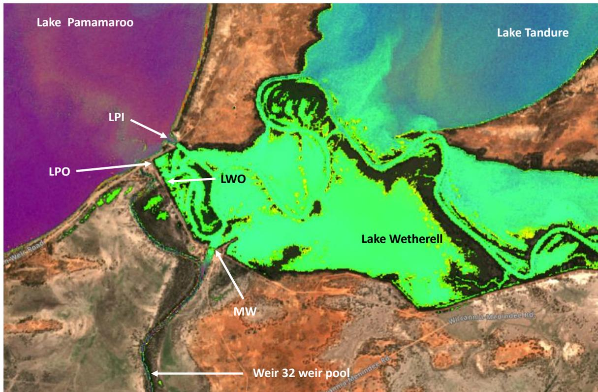
**Figure 2:** False colour Sentinel 2 satellite image of the bottom end of Lake Wetherell and the top end of weir 32 weir pool taken on March 14 processed with the APA script (Pélioiva et al, undated). Algal biomass is shown in green. MW = Main Weir; LPI = Lake Pamamaroo inlet; LPO = Lake Pamamaroo outlet; LWO = Lake Wetherell outlet.
