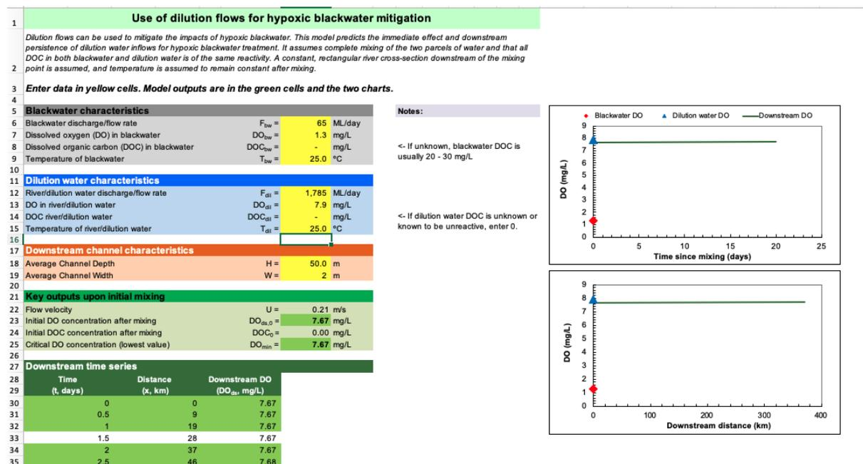
**Figure 9:** Screen shot of the Blackwater Intervention tool dilution model based on actual flows. The dissolved oxygen concentration on mixing is found on line 23
