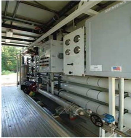
FlexRO reverse osmosis units are installed in mobile water treatment trailers from Siemens Water Technologies.
