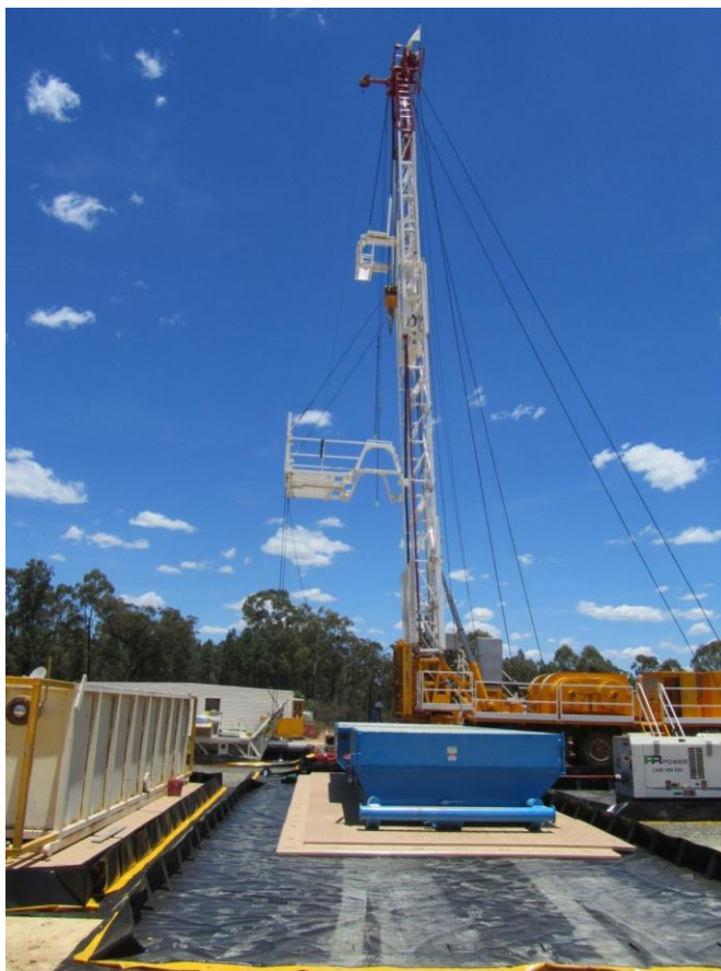
Figure 11. Typical drilling rig used for coal seam gas exploration or production wells. (Source: Santos)
