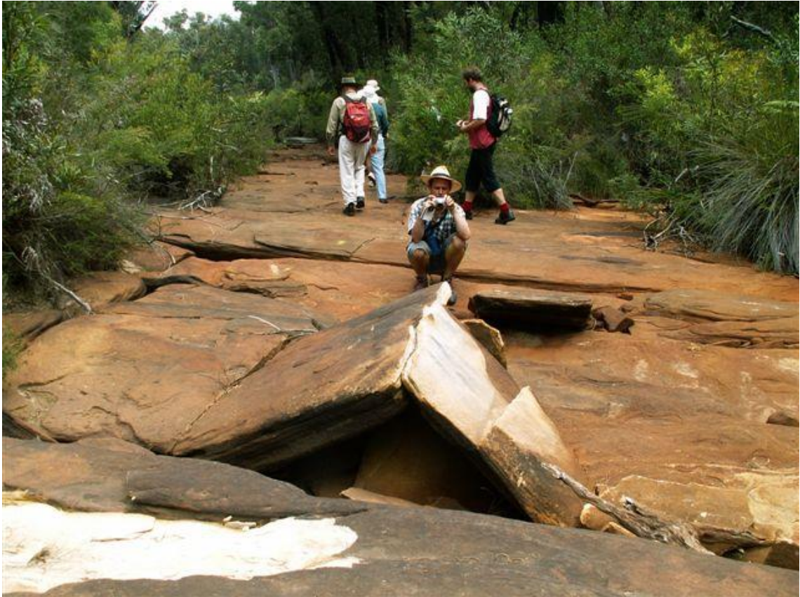
Upsidence effect in a cracked and drained section of Waratah Rivulet
