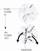
Fracking fluid expands cracks in the rock, releasing oil, which flows back up the well.
