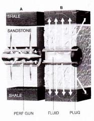
PLUG AND PERFORATION A plug blocks off a section of pipe, and a "perf gun" blasts small holes in the sandstone (A). Fluid is pumped in at high pressure (B), releasing the oil.
