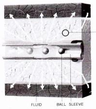
SLIDING SLEEVE Plastic balls are forced down the pipe, pushing open sliding sleeves to expose holes in the pipe. Fluid shoots out through the holes, fracturing the rock.
