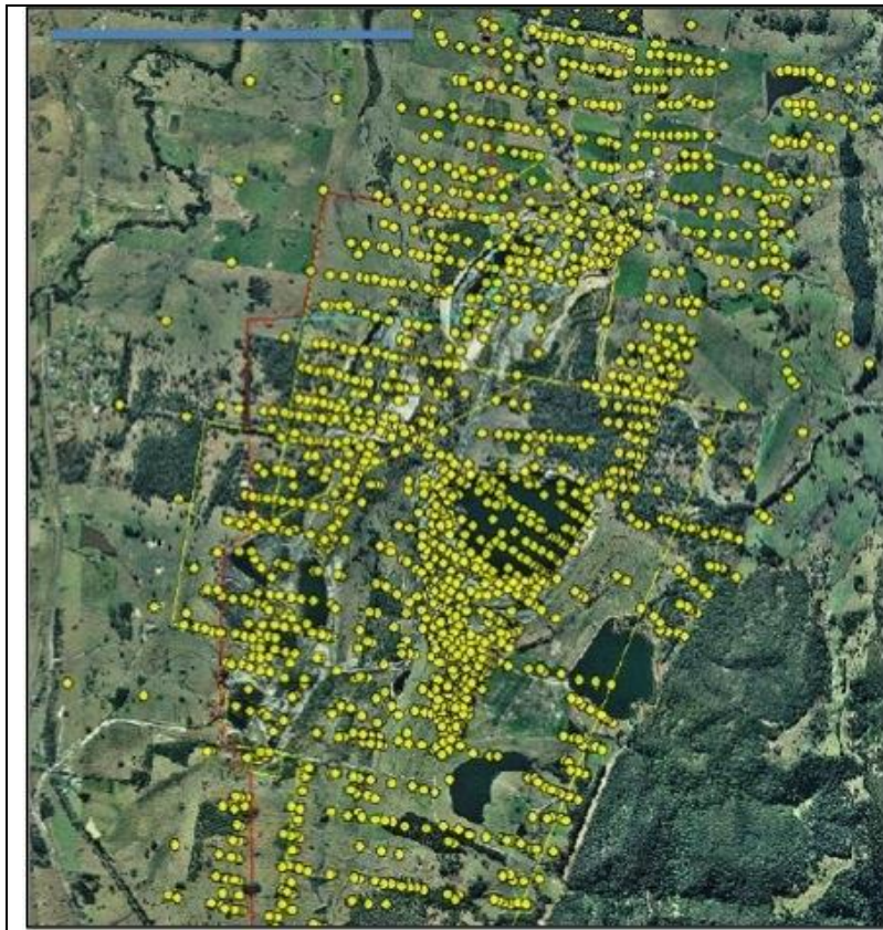
Fig. 3.1. Detail of part of the Gloucester Valley (NSW) showing the locations of all holes >10 m depth drilled within exploration leases.
