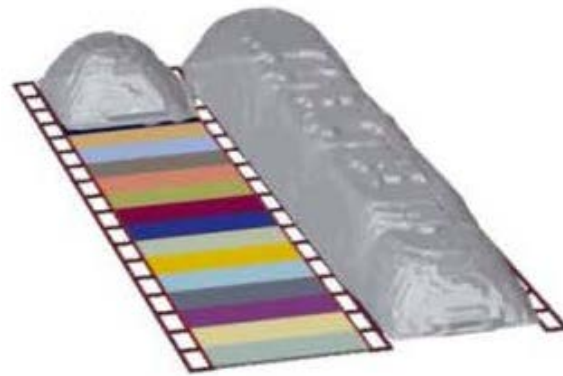
Figure 20. Cut-away view of the developing collapsed zone
