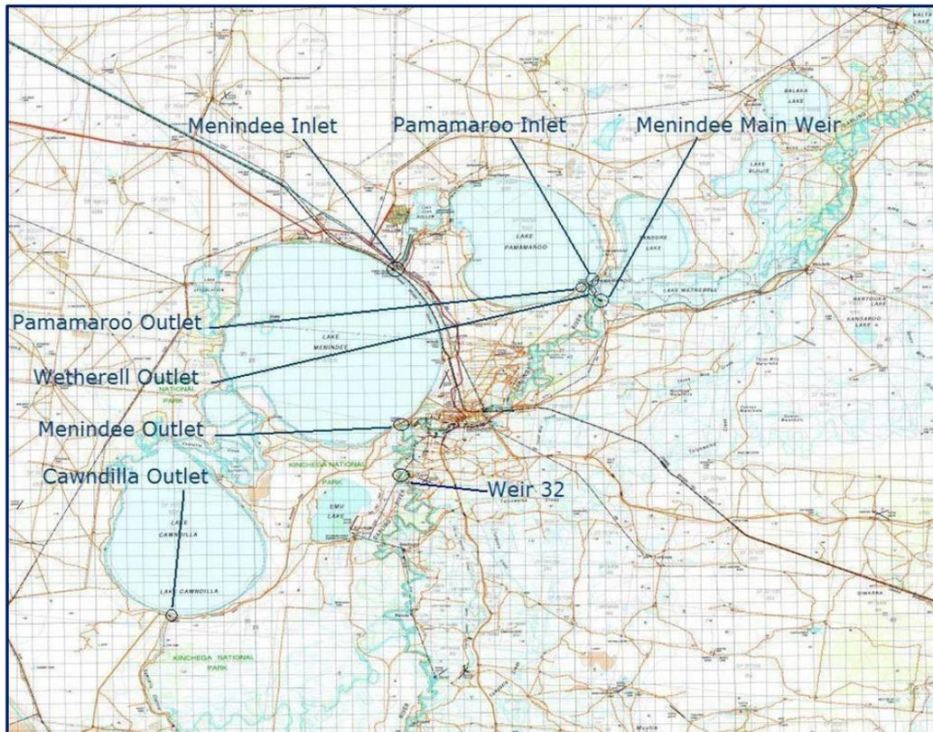
Figure 12- The main structures of the Menindee Lakes scheme. Source - Menindee Lakes Storage Operation and Maintenance Manual, Figure 2, DOC 13/1324
