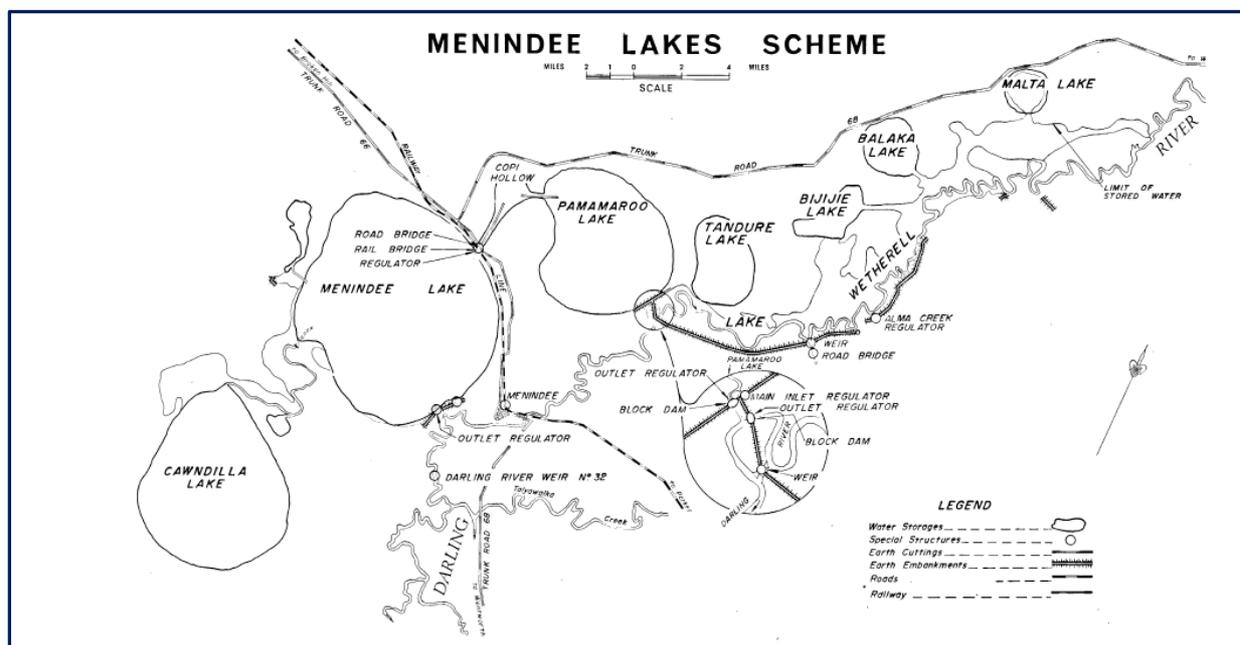
Figure 11- Plan of the Menindee Lakes Scheme. Source Menindee Lakes Storage Operation and Maintenance Manual, Figure 1, DOC 13/13246
