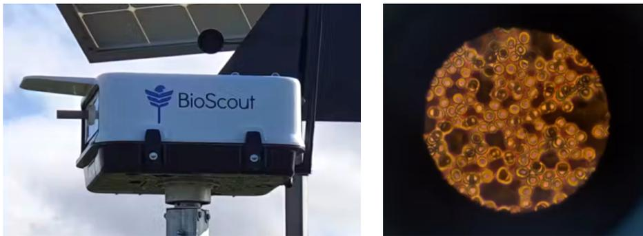
Figure 13: Bioscout's remotely operated microscopy sensor for automated agricultural disease detection. Platforms such as these could potentially enable remote and real-time microscopy analysis of asbestos fibres. Image sourced from [64].
