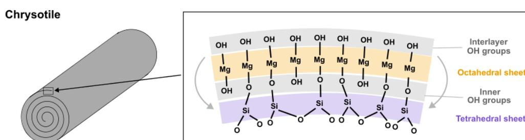
Figure 1: A generic view of a chrysotile fibre, the only serpentine type of asbestos fibre. Its molecular structure consists of Mg-based octahedral and Si-based tetrahedral sheets, which causes the overall structure to 'curl' into spiral structures.
