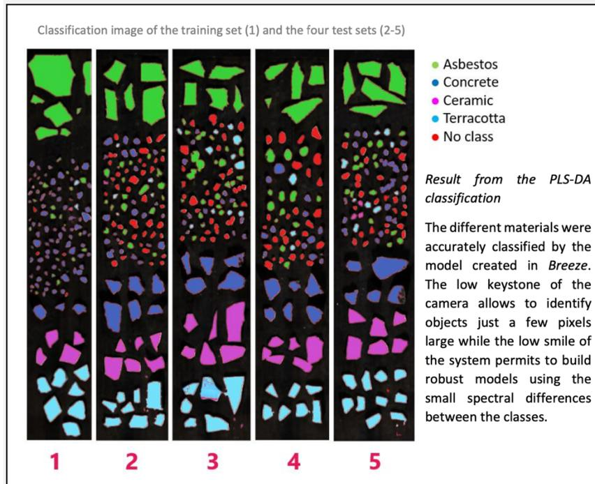
Figure 14: NIR image classification performed on a variety of building materials – identifying whether some of the objects contained asbestos. Image adapted from [52].
