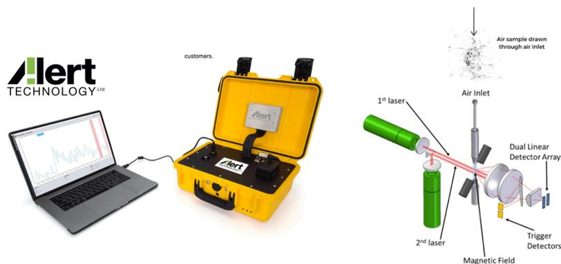
Figure 10: (Left) Alert Technology's ALERT Pro 1000, which uses light scattering from oriented fibres to detect airborne asbestos. (Right) The operating principle of the technology – using magnetic fields to align flowing fibres as they interact with laser light.
