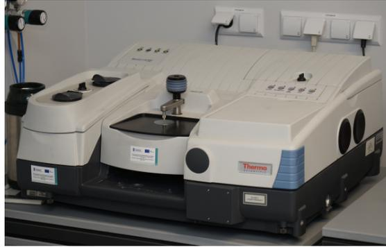
Figure 6: FTIR spectrometer (Nicolet 6700) used for high-quality infrared spectral measurements. This benchtop device allows for relatively simple analysis of asbestos species. Image sourced from [29].
