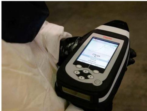
Figure 8: Thermo Fisher Scientific's handheld microPHAZIR AS product – able to identify ACM using NIR spectroscopy. Image sourced from [38].
