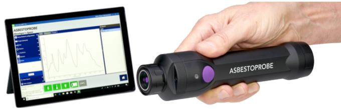
Figure 9: The handheld Asbestoprobe commercialised by Greenwall, which utilises the power of micro near infrared spectroscopy combined with artificial intelligent software. Image sourced from [45].
