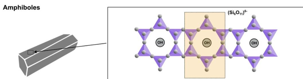
Figure 2: Overall structure of an amphibole fibre – consisting of a double chain of silica tetrahedra.
