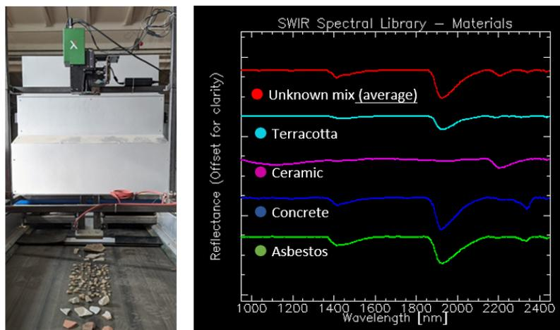
Figure 11: (Left) HySpex Baldur S-384N camera working at ~1 metre working distance to conduct real-time NIR imaging of asbestos samples. (Right) Average SWIR reflectance spectra of five different building materials.
