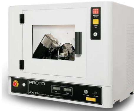
Figure 5: A benchtop power XRD device. Although sample preparation is required to perform accurate measurements, the devices themselves have progressed to be able to be located at waste recycling centres. Image sourced from [25].
