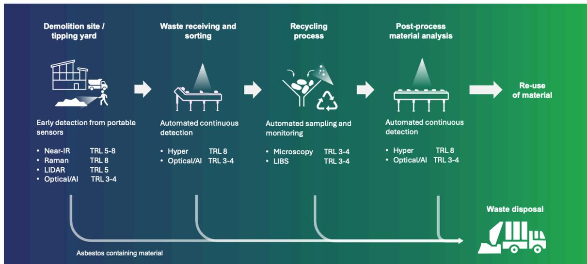
Figure 16: Summary of relevant emerging sensing technologies for asbestos detection, across various points in the recycling process.
