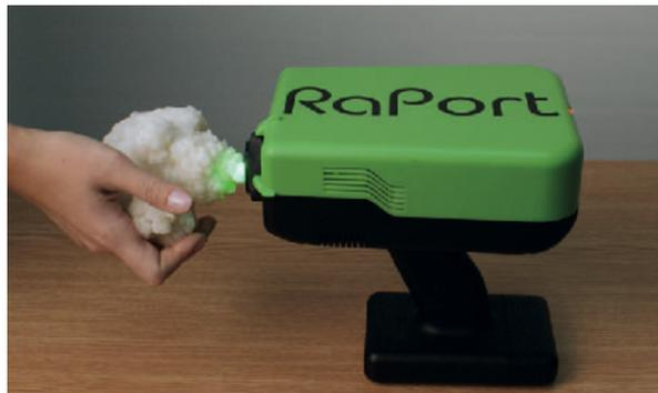
Figure 7: RaPort handheld Raman spectrometer from Enspectr – for in-field diagnostics of minerals. This device uses a green (532 nm) laser to use Raman spectroscopy analyse various minerals, including asbestos. Image was sourced from [34].
