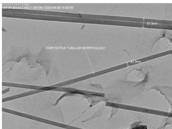
Figure 4: TEM observation of chrysotile asbestos fibre at a display magnification of 150,000x. Image sourced from [76].
