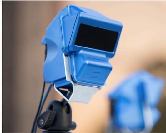
Figure 15: Baraja's LiDAR system initially used in the autonomous vehicle industry. The unit consists of a near-IR laser emitter and detector to produce a point cloud of its surrounding. Image sourced from [66].
