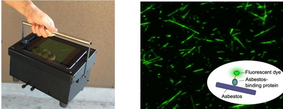
Figure 12: Shining the light on asbestos – Hiroshima University’s developments for a robust and portable fluorescence microscope for on-site asbestos detection. Image adapted from [59].
