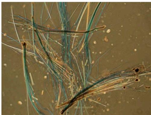
Figure 3: Crocidolite fibres viewed under PLM, showing interference colours (birefringence) and parallel extinction at x125 magnification. Image was sourced from [14].
