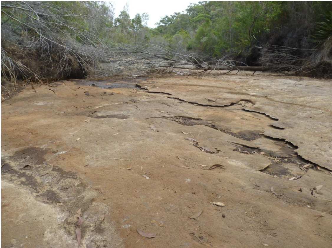
Short distance ‘upstream’ from the crack at the southern end of Pool N into which water was draining, February 13 2014. A layer on the river bed has been pushed upwards (upsidence).
