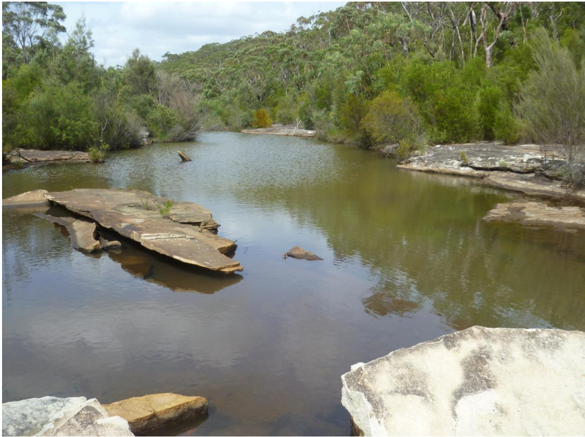
Green water looking upstream along Pool F from the edge of Rockbar F (WRS4). Note the large displaced bedrock fragments from the subsidence impacted river bed.
