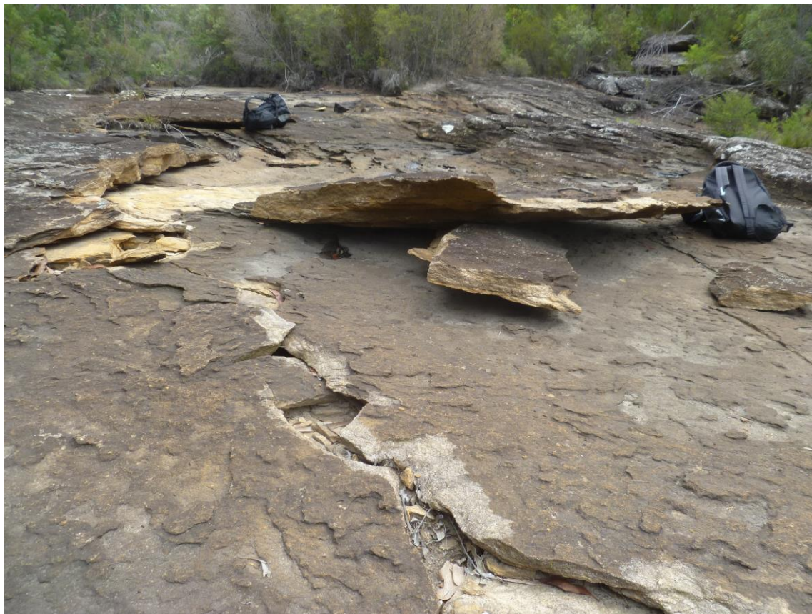
Cracking and uplifting (upsidence) to the east across the surface of Rockbar N. The extent of the cracking has increased since October 2012.
