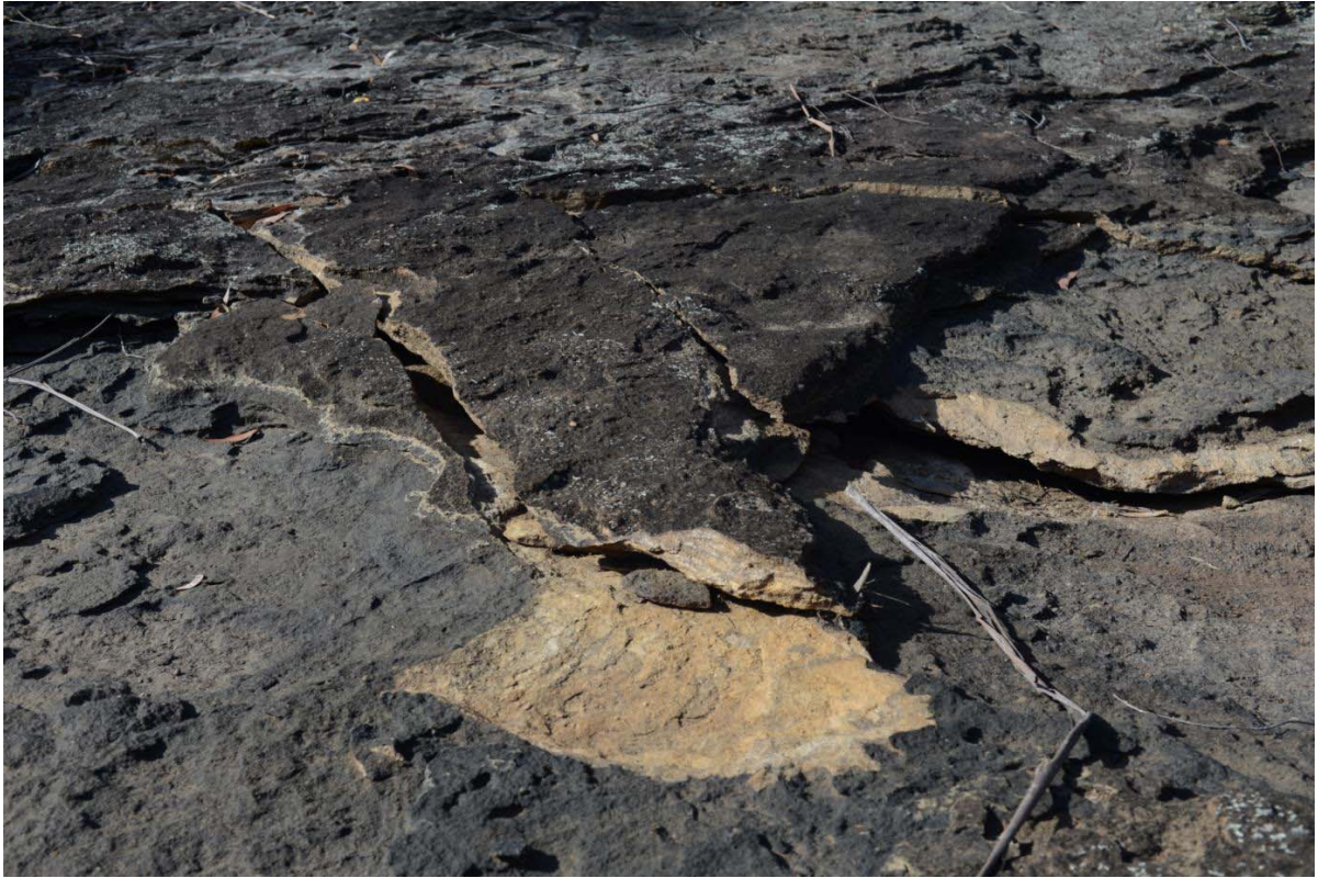
Upsidence impacts on the surface of the shattered rockbar Rockbar N (WRS5)
