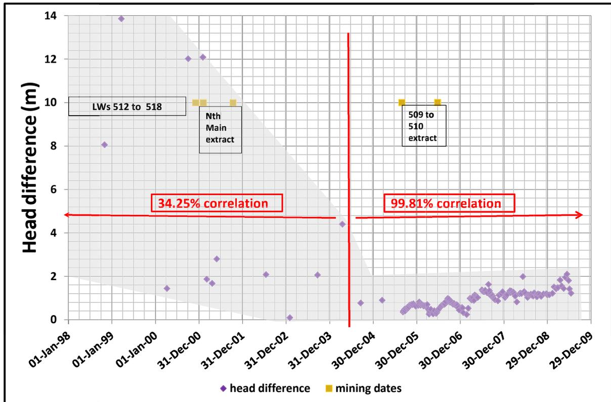
Figure 15 Difference in water levels in Cataract Reservoir and Piezometer 514
