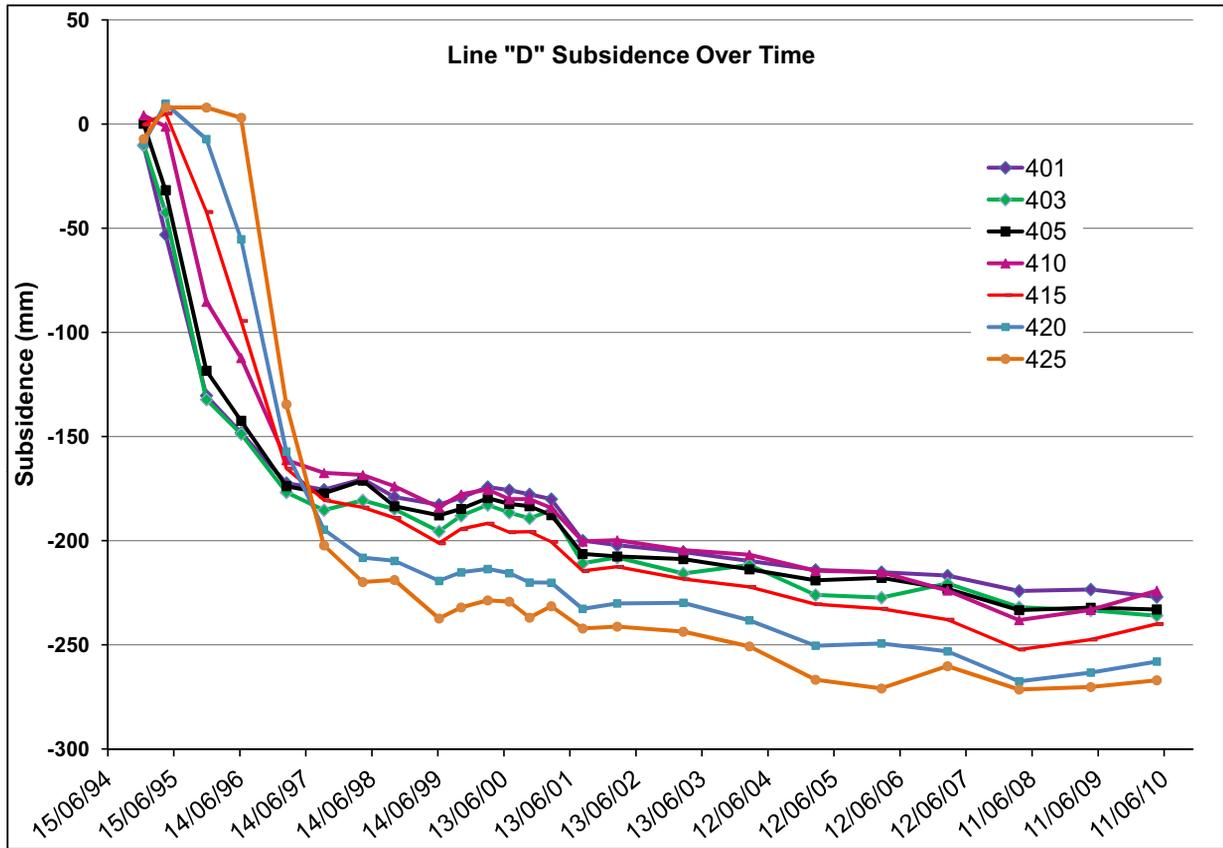
Figure 10 Time series of subsidence at various pegs along Line D-D
