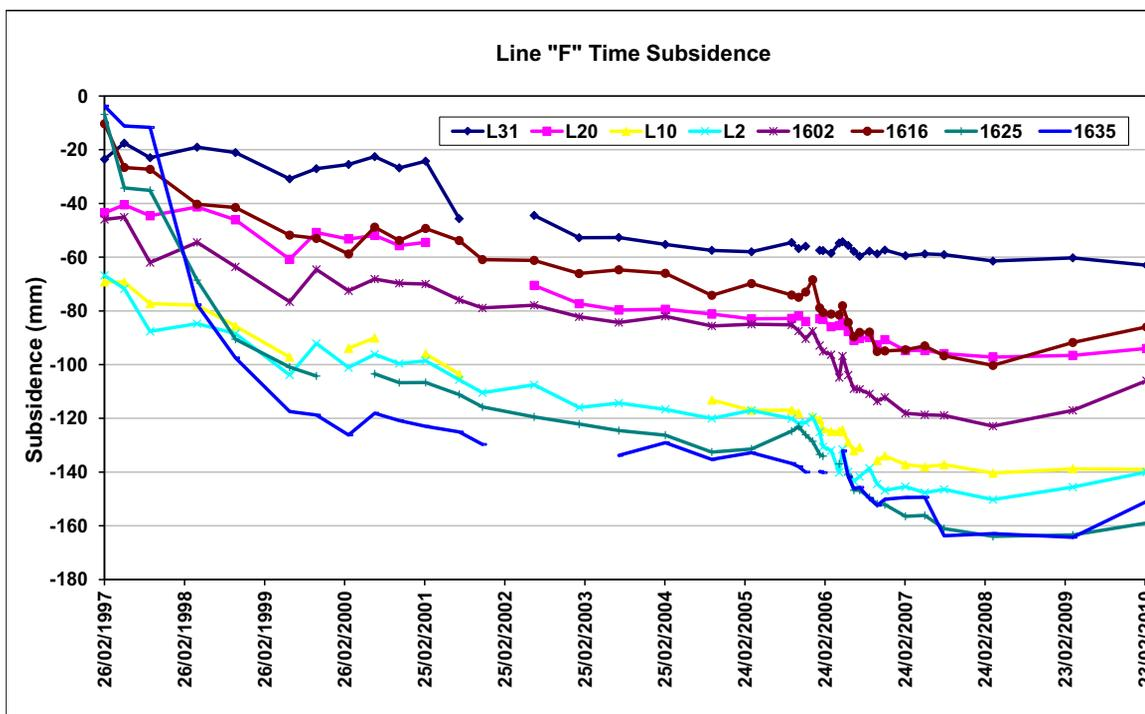
Figure 9 Time series of subsidence at various pegs along Line F-F
