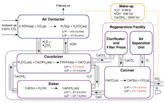
DAC utilises big fans to induce air flow through a CO2 separation process that uses reversible chemical and physical sorbents to trap the gas. Chemical sorbents include aqueous hydroxides (like NaOH, KOH, Ca(OH)<sub>2</sub> etc.) and carbonate forming solvents (CaO)<sup>256</sup>. These chemicals bind the CO<sub>2</sub> on interaction with air and can then be later regenerated by thermal heating to release CO<sub>2</sub> (**Figure 43**).
