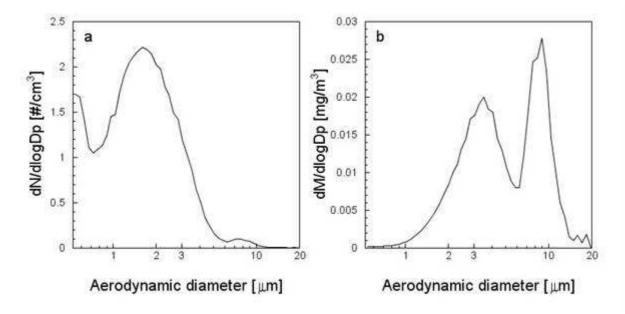
Figure 2 Size distribution of a) number and b) particle mass of particles generated from the resuspension of road dust in experimental conditions (Civiš and Hovorka 2010).
