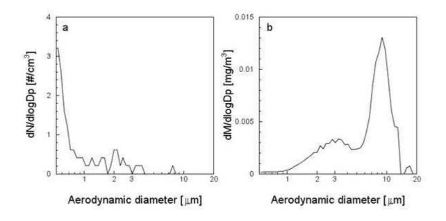
Figure 1 size distribution of a) number and b) particle mass of particles generated from the resuspension of brown coal dust in experimental conditions (Civiš and Hovorka 2010).
