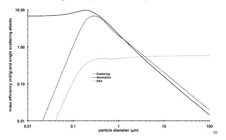
Figure 4 Mass scattering and absorption efficiency as a function of particle diameter for a spherical BC particle with a density of 1.8 g cm<sup>-3</sup> calculated from theory at 550 nm. From Moosmuller et al (2009)
