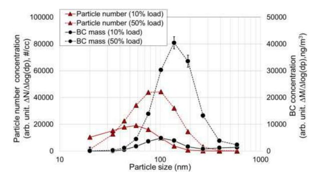
Figure 3 Particle number and black carbon mass size distributions from diesel engine emissions under experimental conditions (from Ning et al., 2013)
