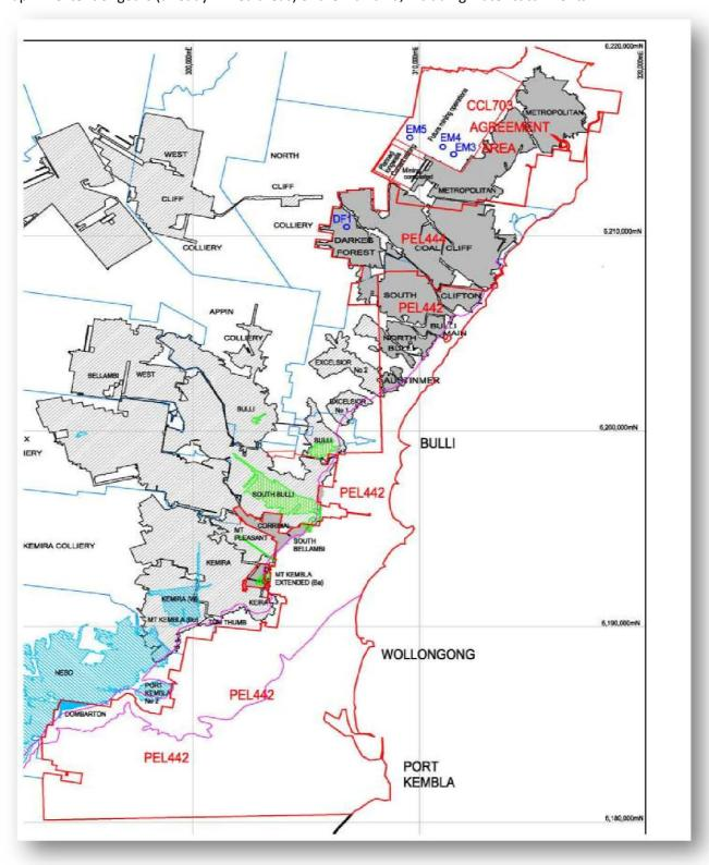
Map 2 – Map of Westcliff Colliery and surrounds, to the west of Apex Illawarra PEL's. Showing intensity of exploration boreholes drilled, including in water catchments, and being indicative of other mined areas.
